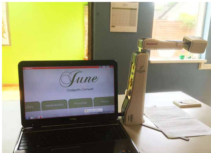
Aumax-S with iZoom used in a copy typing situation using distance viewing to the computer
